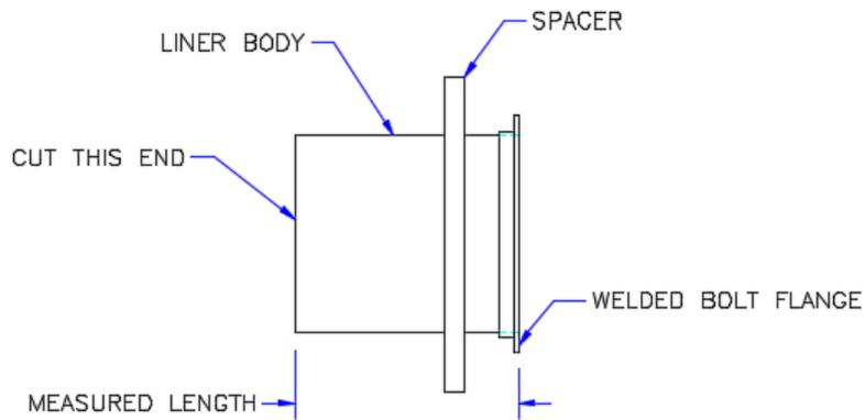
Figure 3: Cut the Liner Body to the measured length between adjacent sections.
