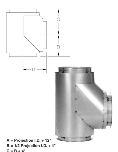
These formulas may be used to determine boot tee dimensions with reduced projections.
